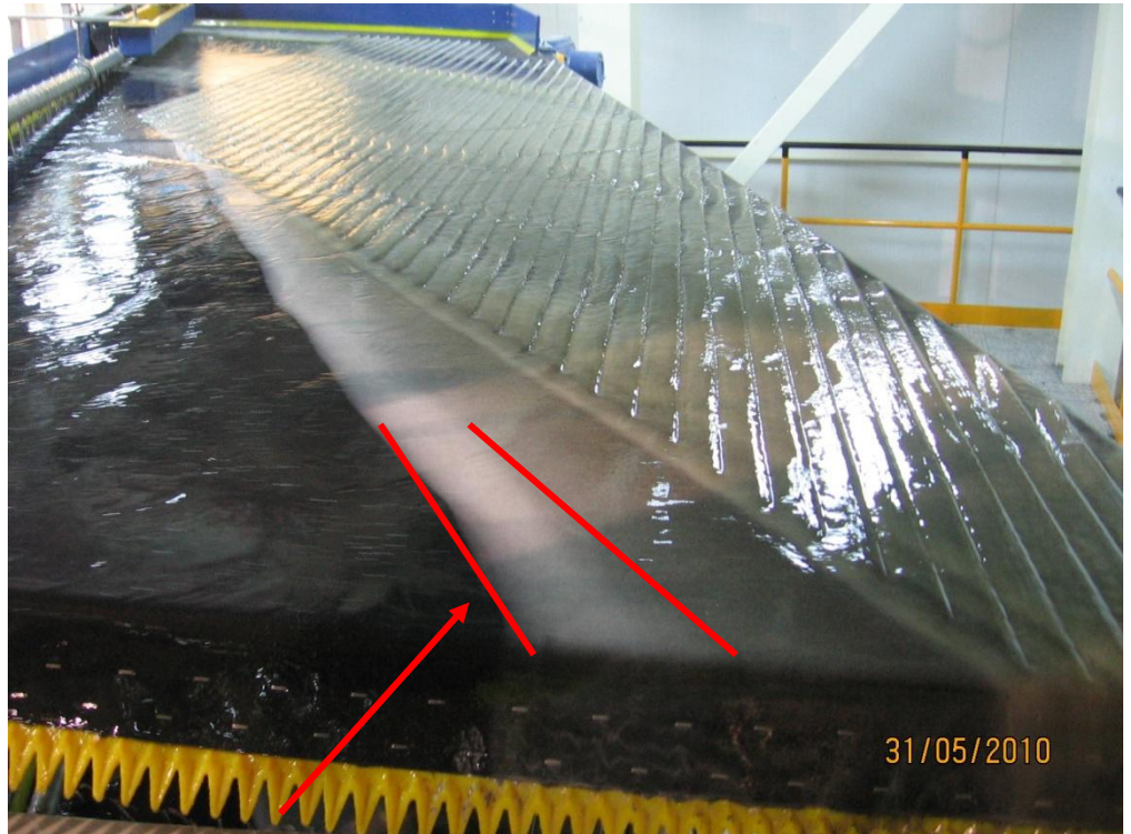
Figure 3: Concentrate production on tables following recommissioning
