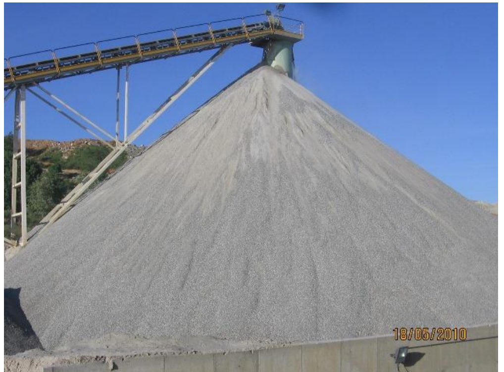
Figure 4: Crushed ore stockpiled ready for milling
